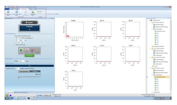
You can move, minimize, or hide the Experiment Explorer, the Collection Panel, and the Instrument Panel.
