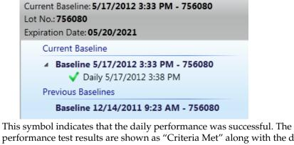
performance test results are shown as "Criteria Met" along with the date and time of the run.
