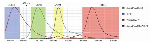
Each dye emits with a characteristic emission spectrum that is specific for the fluorophore: Alexa Fluor<sup>®</sup> 488 dye has a maximum around 520 nm, R-PE at about 575 nm, Pacific Blue<sup>™</sup> dye at about 454 nm, and Alexa Fluor<sup>®</sup> 647-R-PE dye at about 666 nm. The teal line represents the laser excitation wavelength of an argon ion laser (488 nm).
