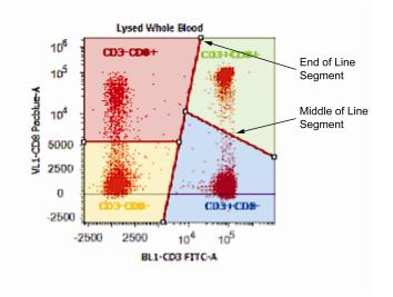
Grabbing the middle of a line segment allows for the independent movement of each arm.
