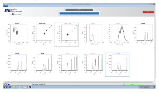
The progress bar provides an ongoing update during the run and displays the steps of the performance test.
