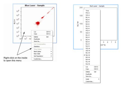
Right-click on the plot and select **Customize** to open the Customize Plot dialog box. Customize Plot dialog box has six tabs: General, X Axis, Y Axis, Samples, Gates, and Back Gates.
