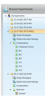
Experiments are groups of specimens and samples that share common Workspaces, instrument settings, and compensation settings.
