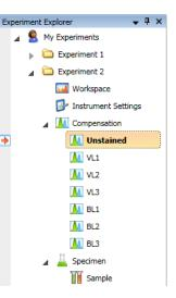
IMPORTANT! Once you click **Record** on any of the compensation controls within the compensation setup, the Instrument Settings for all fluorescent channels will be grayed out and cannot be changed. It is critical that you optimize voltages prior to recording any sample or any compensation controls.
