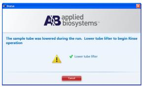
If the tube lifter is down, Rinse operation automatically starts. If the tube lifter is up, lowering the tube lifter initiates the Rinse.
