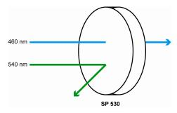
**Dichroic Mirror** *Dichroic mirrors,* also called "reflective," "thin film," or "interference" filters, are produced by coating a glass substrate with a series of optical coatings. Dichroic filters usually reflect the unwanted portion of the light and transmit the remainder.
