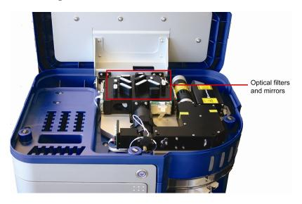
2. Remove the optical holder containing the appropriate filter or mirror.
