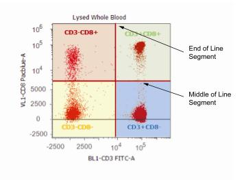
In a Flexible Quadrant Gate, the lines that demarcate the populations of interest do not form right angles, as shown in the example below.
