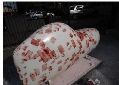
Top: Plug design; used to create carbon fiber fairing.
