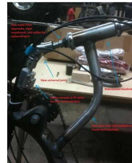
This year's steering system for our bike is new; using a Universal Joint. This was done to minimize the needed clearance for the driver to turn, while preserving the necessary turning radius.
