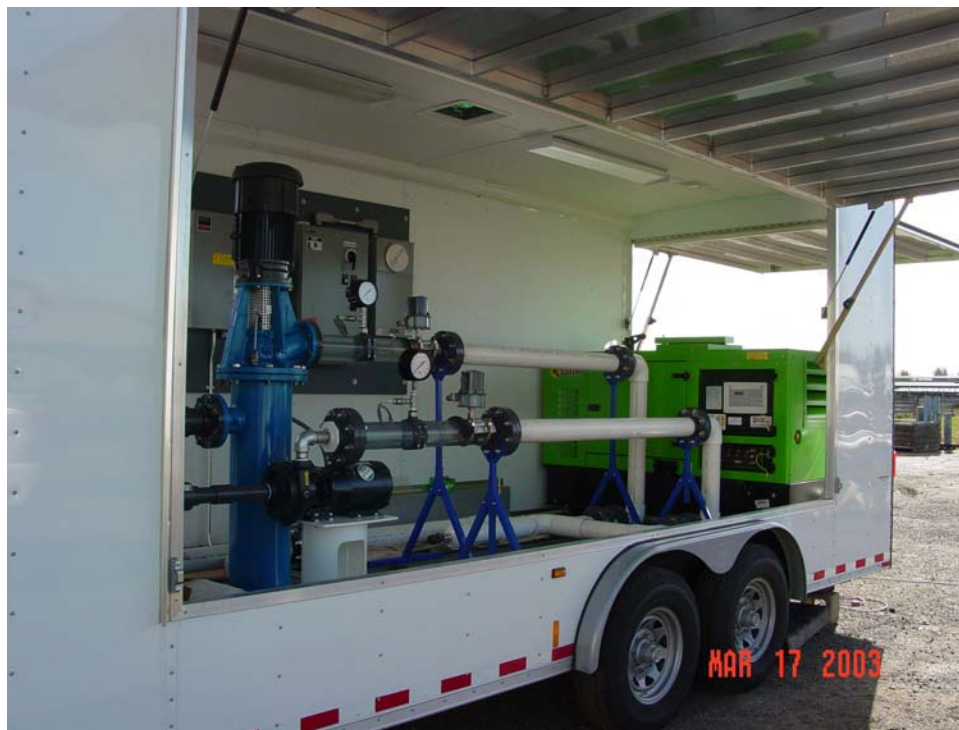
Figure 1 – View of Mobile Education Center showing vertical turbine and horizontal centrifugal pumps and the generator powering the pumps.
