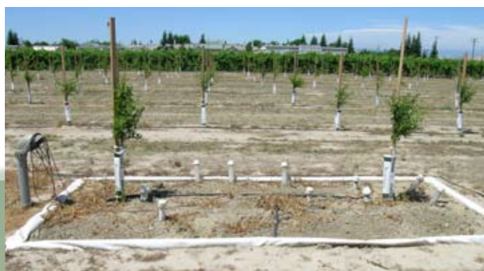
Photo shows one of two weighing lysimeters that will record water use of two trees.
