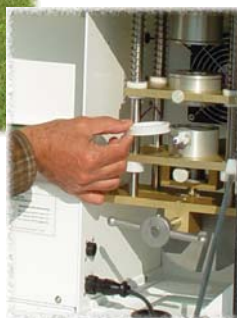
Fresno State research associate Shawn Ashkan displays one of six air sampling units recently purchased for air emissions study. The sampler uses a small electric motor to draw air in through the stack on top, then collects particles in the filter being shown inserted, at right.
