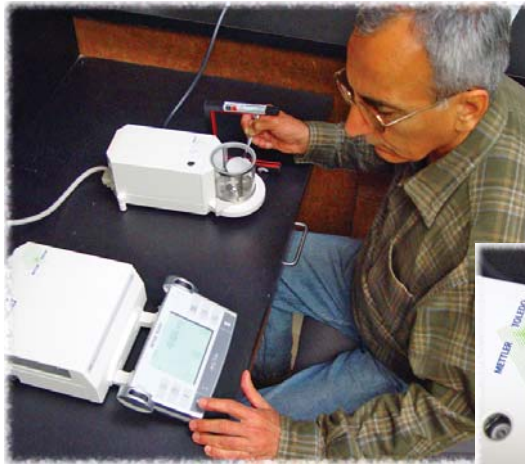
Fresno State research associate Shawn Ashkan uses a Mettler-Toledo model MX5 micro scale (top unit in left photo) to weigh collected particulate matter. Unit on his left calculates weight and other information.
