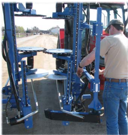
Oxbo viticultural specialist Greg Berg adjusts a California-Sprawl head of a mechanical pruner. The head features flat, circular rotary bar pruners in the center and vertical sickle bar pruners along the outside of the head.
