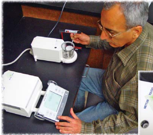
Fresno State research associate Shawn Ashkan uses a Mettler-Toledo model MX5 micro scale (top unit in left photo) to weigh collected particulate matter. Unit on his left calculates weight and other information.
