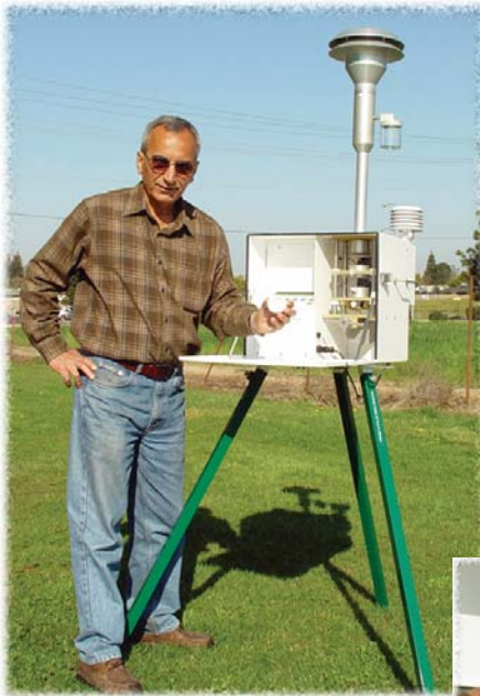
Fresno State research associate Shawn Ashkan displays one of six air sampling units recently purchased for air emissions study. The sampler uses a small electric motor to draw air in through the stack on top, then collects particles in the filter being shown inserted, at right.
