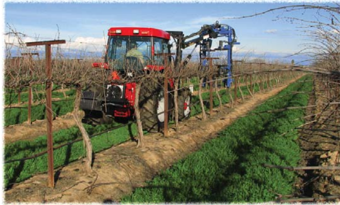
Cabernet Sauvignon grapevines at the Fresno State University Farm are mechanically pruned during recent trials featuring new pruning and thinning heads developed by Oxbo International.
