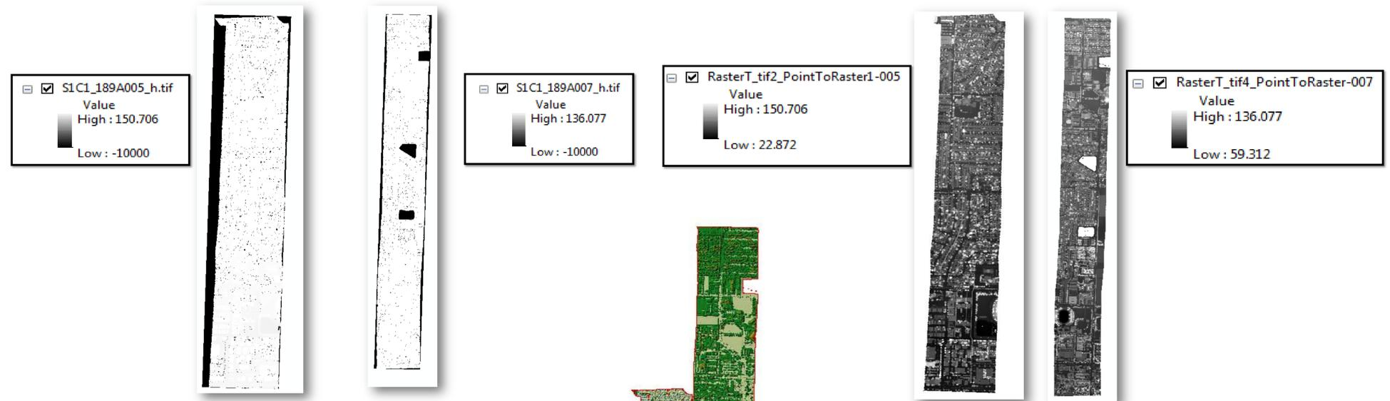
The images above represent the GeoTiff data being used for the analysis. The areas with black represent the "NULL" values, which were set to be -10000. In order to properly compare the data, these values had to be removed.
