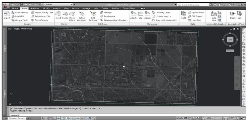
The images above depict the process to create a Google Earth surface in 2012 Civil 3D. The first figure shows the view in Google Earth. It had to be oriented with in plan view, in order to properly represent the area when creating a surface. The second image shows the surface created in 2012 Civil 3D.
