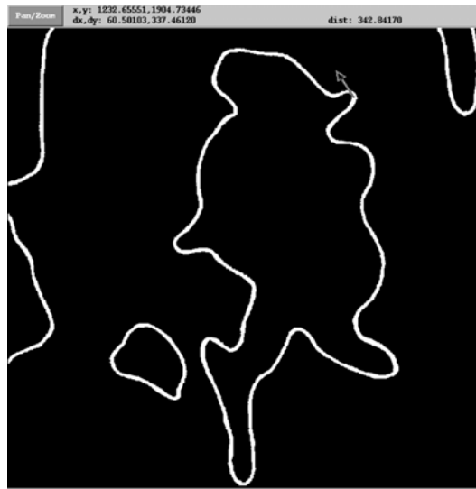
Figure 5.14 Semiautomatic tracing starts at a point (shown with an arrow) and traces all lines connected to the point.
