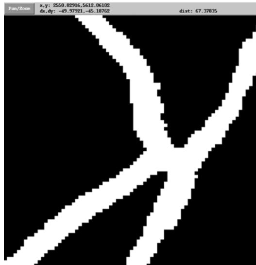
Figure 5.15 The width of a raster line doubles or triples when lines meet or intersect.
