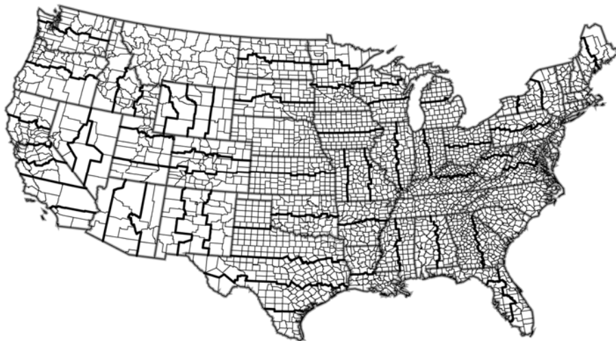
Figure 2.14 SPC83 zones in the conterminous United States. The thinner lines are county boundaries, and the gray lines are state boundaries.
