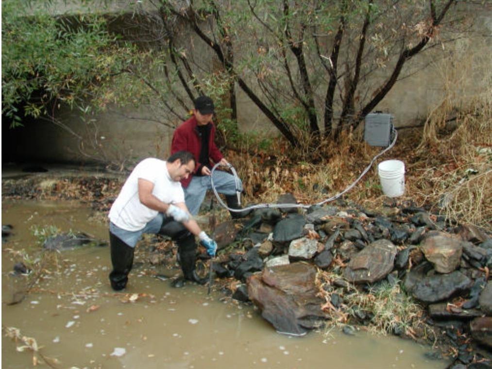
Graduate student Jorge Baca (front) and Zili He are installing a storm water sampler to automatically take water samples during the first flood in Coarsegold Creek (CGC010).
