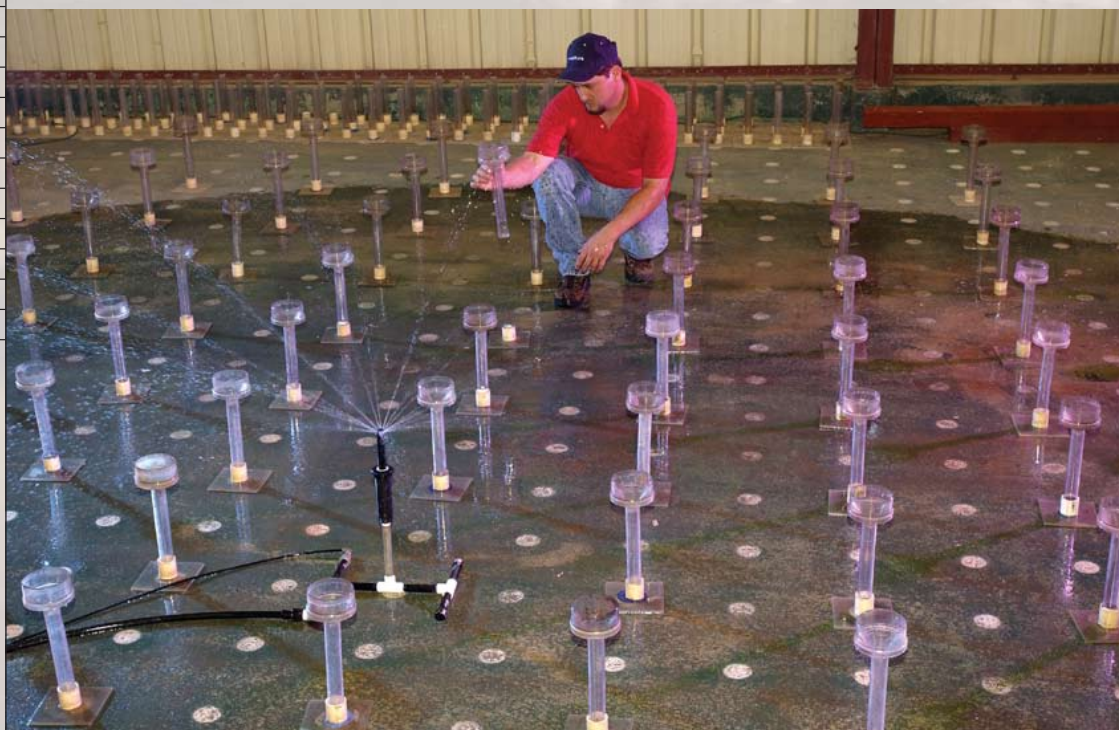
Gonsalves reads catchments on a full grid sprinkler distribution test.
