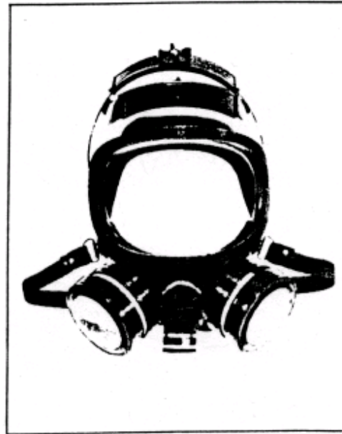
Figure 6 — (a) Half-mask facepieces may be used to protect against substances that do not irritate the eyes and that are not absorbed through the skin. (b) Full-facepiece masks should be used to protect employees against eye irritations and excessive exposure to a material through skin absorption.
