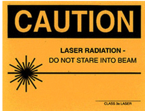
ANSI sign to mark doors to laser labs with Class 3a lasers.
